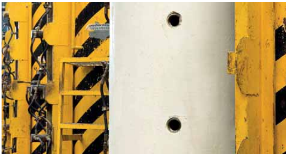
Rigid, mould-injected PU insulating material
