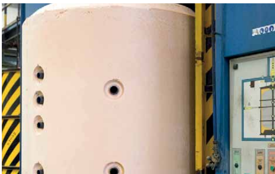
Rigid, mould-injected PU insulating material.
