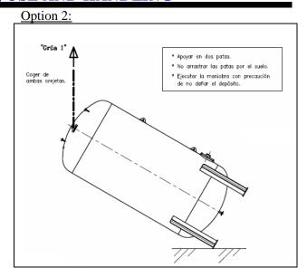
In both cases, the angle of the slings/chains on the bottom lugs must not exceed 60°.
