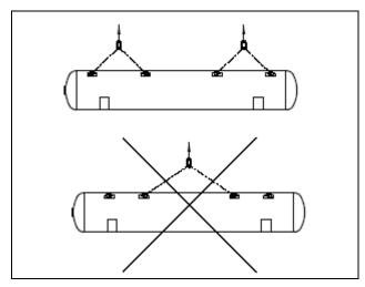
• If the vessel has 8 lifting lugs under the apex (two at either end and four in the middle), it should be hoisted as shown in the illustrations.
