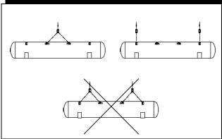
Other devices that do not make use of the lugs, such as forklift trucks or girth belts around the vessel, can be used to lift the vessel providing they adhere to the relevant safety regulations. In such cases, special care must be taken to protect the vessel coating.
