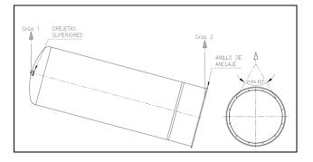
The same as for vessels on feet, the angle of the lifting slings/chains through the bottom lugs must not exceed 60° (see top illustration).
